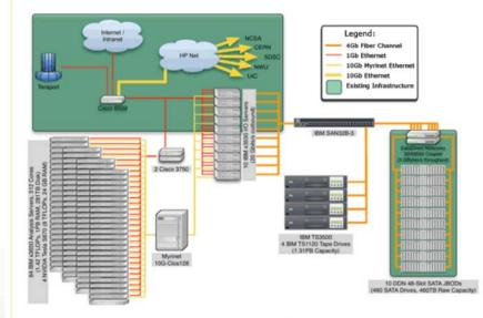
System diagram of the PADS environment, showing links to other resources.
