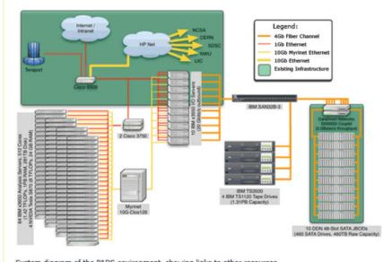
PADS is a petabyte (1015-byte)-scale online storage server capable of sustained multi-gigabyte/s I/O performance, tightly integrated with a 9 teraflop/s computing resource and multi-gigabit/s local and wide area networks. Its hardware and associated software enables the reliable storage of, access to, and analysis of massive datasets by both local users and the national scientific community.
