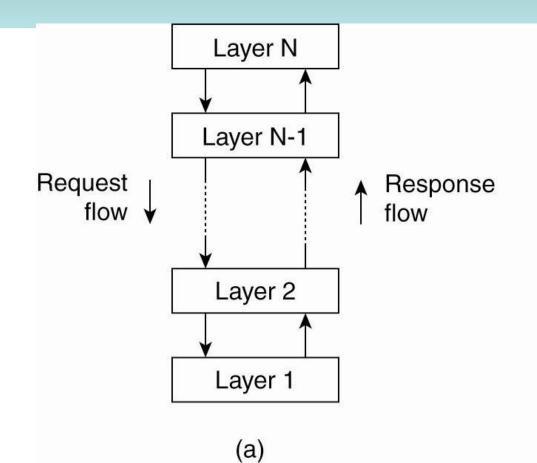
Components are organized in a layered fashion where a component at Layer  $L_i$  is allowed to call components at the underlying layer  $L_{i-1}$
