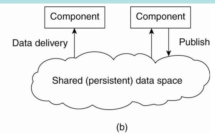
Processes communicate through a common repository; When combining with event-based architectures, it is also known as shared data spaces
