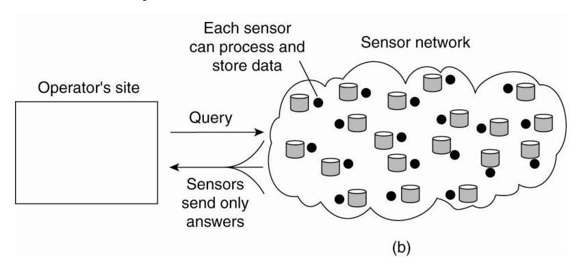
Organizing a sensor network database, while storing and processing data ... or (b) only at the sensors.
