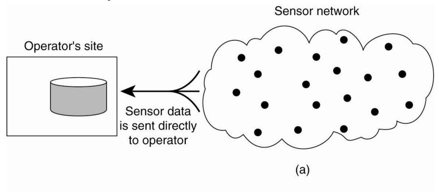
Organizing a sensor network database, while storing and processing data (a) only at the operator's site or ....
