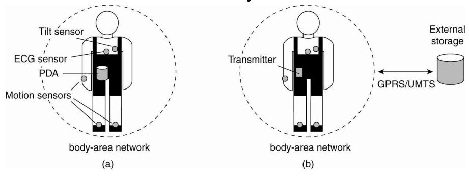
Monitoring a person in a pervasive electronic health care system, using (a) a local hub or (b) a continuous wireless connection.
