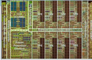
IBM Cell: 8 slave cores + 1 master core, 2005
