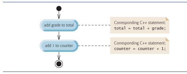
**Fig. 4.2** | Sequence-structure activity diagram.
