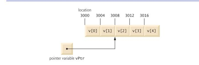
**Fig. 8.17** | Pointer vPtr after pointer arithmetic.
