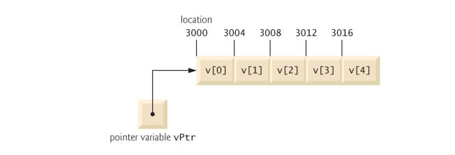
**Fig. 8.16** | Array v and a pointer variable int \*vPtr that points to v.
