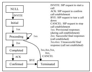
Figure 5: Modeling the SIP protocol state machine
