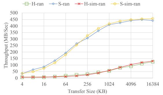
Fig. 5: Random Write Performance Comparison between Real System and HPIS3
