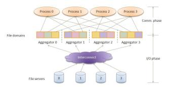
Figure 2. Collective I/O and Two-phase Implementation. The two-phase implementation has a communication phase to exchange data between I/O client processes and aggregators and an I/O phase to carry out I/O requests via aggregators collectively.
