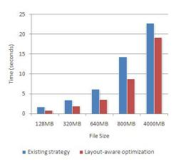
Figure 8. Layout-Aware Collective I/O Optimization with Synthetic Benchmark Testing
