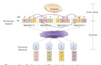
Figure 5. Collective I/O with Layout Awareness. This new strategy rearranges the partitions of file domains and the requests of aggregators to be physically contiguous as much as possible. This strategy exploits better locality, reduces contention and achieves better I/O performance.
