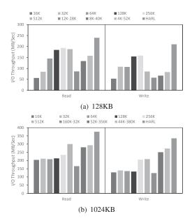
Fig. 9. Throughputs of IOR with various request sizes
