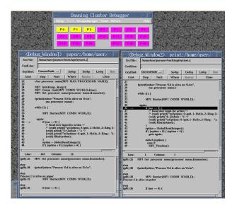
Figure 4 The DCDB views for debugging MPI programs
