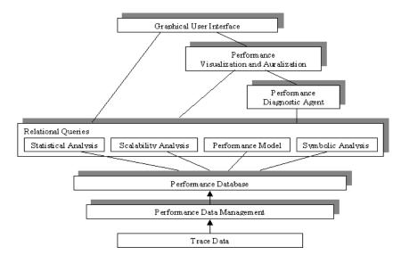
Figure 2.1 Design framework of PDRS
