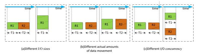
Figure 1. Two I/O requests R1 and R2 are served by an I/O system in 6 different cases. In each case, each request is represented by a rectangle, of which the length means the I/O completion time and the height means the I/O request size. Each subfigure presents two I/O access cases for comparison.
