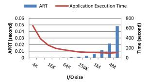
Figure 8. ARPT and application execution time with various I/O sizes in SSD environment.
