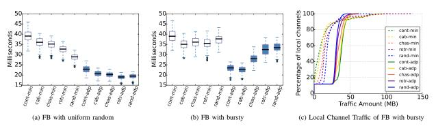
Fig. 10: Communication time and local channel traffic of FB with background traffic.
