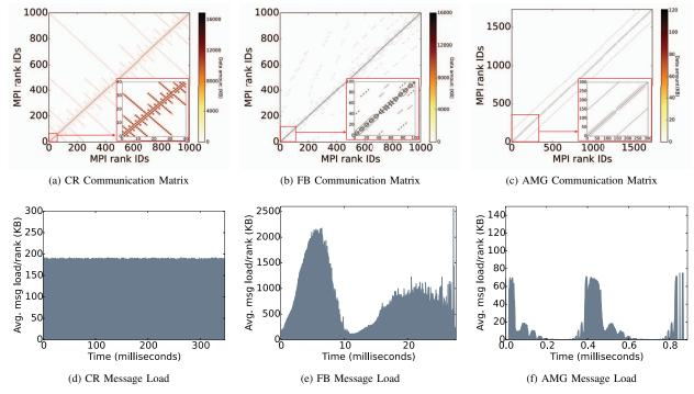
Fig. 2: Communication matrix (top) and message load per rank (bottom) for selected applications. In communication matrix plot, the label of both the x- and y-axes are the index of MPI ranks; the legend bar on the right indicates the message transfer amount between ranks. (CR = Crystal Router, FB = Fill Boundary, AMG = Algebraic MultiGrid)
