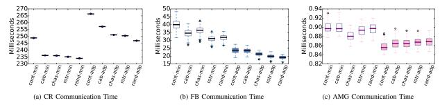
Fig. 3: Application communication times under different placement and routing configurations.
