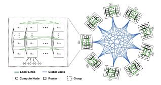
Fig. 1: Overview of the dragonfly system configuration
