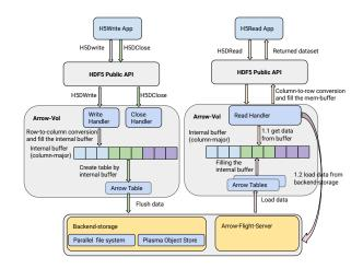
Fig. 2. Internal workflow in Arrow VOL Connector
