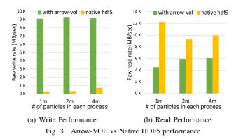
reason is that native hdf5 needs to flush data into the file system when executing the *H5write()* operations while the data is saved in memory when using Arrow Vol connector. Figure 3(b) shows the read performance with arrow-vol and without hdf5. We can see that the performance of without arrow-vol far exceeds that of with arrow-vol. That's probably because the test scale is small and part of the data has been cached in memory.
