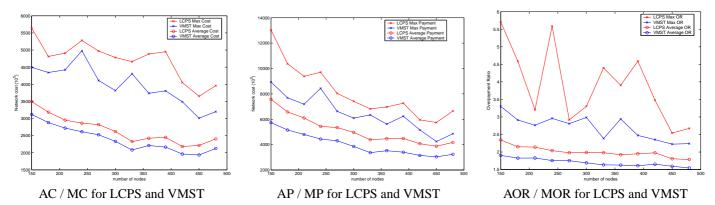
Fig. 5. Results when the number of nodes in the networks varies from 150 to 320 for LCPS and VMST. Here, we fix the transmission range to 300 ft.
