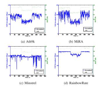
Fig. 6: RA UDP throughput with dynamic transmit powers.
