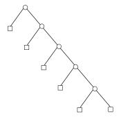
Figure 2: An extremely imbalanced full binary tree.
