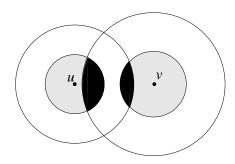
Figure 8: The black region denotes I(u, v). Here the lightly shaded disks denote the transmission regions and the white larger disks denote the interference regions.
