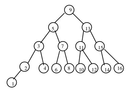
If we insert the key 1, we must move every single node in the tree to rebalance it, taking  $\Theta(n)$  time.
