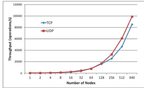
Figure 1: ZHT throughput on SiCortex
