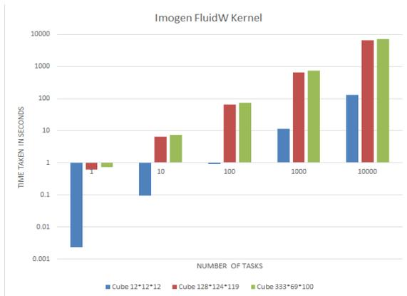
The above graph plots the time taken to complete Imogen FluidW tasks by GeMTC. As usual the size of data has direct impact on the time taken to complete the number of tasks. We also observe that there is almost linear increase in time taken to complete tasks with rise in number of tasks. Also to be noted that data size provided to GeMTC is 181.439 MB for 128\*124\*119 (because the number of equation parameters are large), 220.634 MB for
