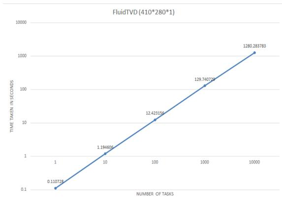
The above graph plots the time taken to complete Imogen FluidTVD tasks by GeMTC. As usual the size of data has direct impact on the time taken to complete the number of tasks. We also observe that there is almost linear increase in time taken to complete tasks with rise in number of tasks. Also to be noted that data size provided to GeMTC is 10.104688 MB for 410\*280\*1 (because the number of equation parameters are large). This was the data set provided by Erik the original writer of Imogen.
