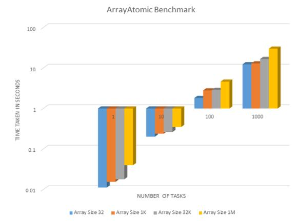
ArrayAtomic plot for varying data-size and its impact on turnaround time for completing a given number of tasks. Please note that it is for comparing data-size only hence there is only 1 task on GEMTC queue at a time. We see linear rise in time taken to complete jobs with increment in number of tasks also in each set the time taken by larger data-size array is more when compared to task with less data-size. This is all expected behavior.
