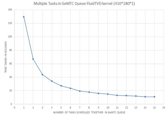
This benchmark analyses impact of scheduling multiple FluidTVD tasks in GeMTC queue. The total number of tasks scheduled is 1000, the explanation is same as of ArrayRotate.
