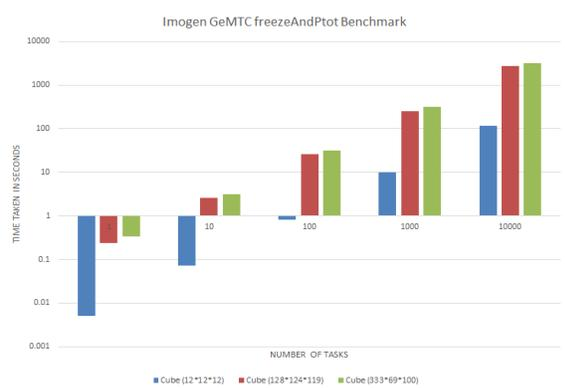
The above graph plots the time taken to complete Imogen freezeAndPtot tasks by GeMTC. As usual the size of data has direct impact on the time taken to complete the number of tasks. We also observe that there is almost linear increase in time taken to complete tasks with rise in number of tasks. Also to be noted that data size provided to GeMTC is 90.778 MB for 128\*124\*119 (because the number of equation parameters are large). 110.344 MB for 333\*69\*100 and 84.136KB for 12\*12\*12.
