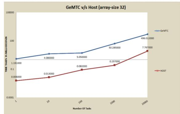
This plot tells us that CPU only code beats the GEMTC code in performance. This is attributed to the fact that the data-size is too small because of this the GEMTC overhead of moving data Host to device and back dominates the processing advantage given by CUDA cores.
