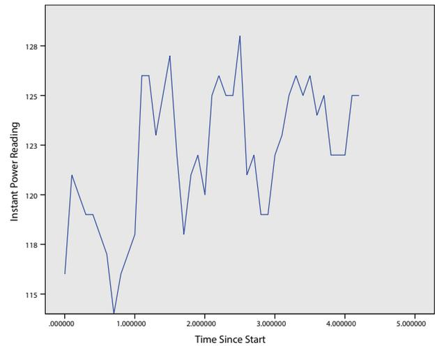
Fig. 6. Sleep workload on Xeon Phi utilizing GeMTC. Shows less chaotic pattern as opposed to directly offloading sleep instruction to Mic, however the power consumption still has a range of about 15 Watts.
