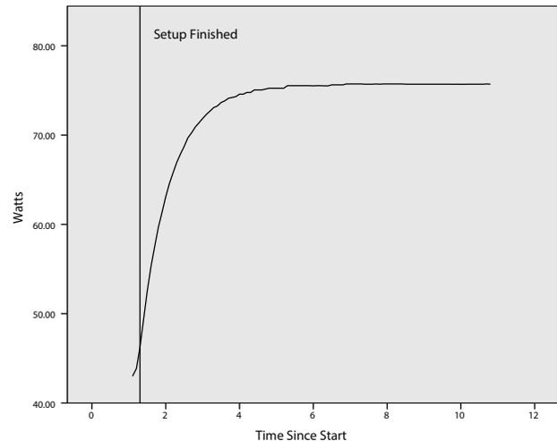
Fig. 1. Shows sleep MTC workload using GeMTC. After GeMTC is fully setup, the power consumption continues to slowly increase over the course of a few seconds leveling off near the 75 Watt mark.
