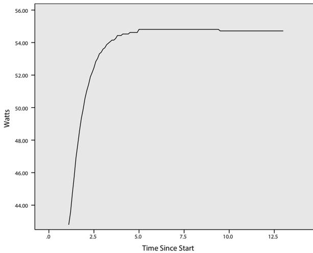
Fig. 2. Standard sleep (without using GeMTC) on GPU. Shows similar power curve as the GeMTC version but maximum power consumption is about 20 Watts less.
