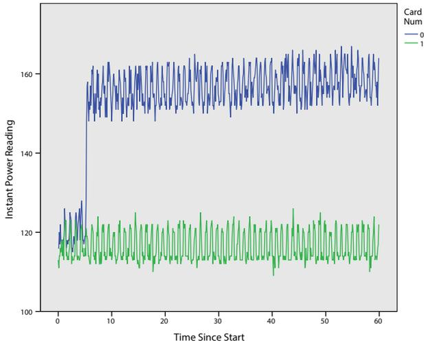
Fig. 8. Vector add workload on Xeon Phi utilizing GeMTC. Shows similar pattern to directly offloading the workload and still exhibits up-down power consumption pattern. Total power consumption is about 10 Watts higher than with traditional offloading and the total runtime is about 10 seconds longer.
