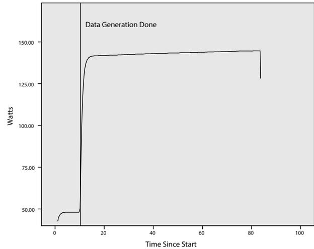
Fig. 3. Vector add implemented with vanilla CUDA. At beginning shows power ramp up present in both sleep tests. After data generation power rapidly increases to a level of about 140 Watts and stays there for the remainder of the computation.
