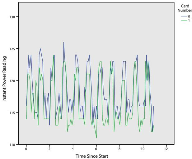
Fig. 5. Sleep workload on Xeon Phi without GeMTC. Shows chaotic power consumption for both cards installed in machine. Range is about 10 Watts between highest and lowest power consumption.
