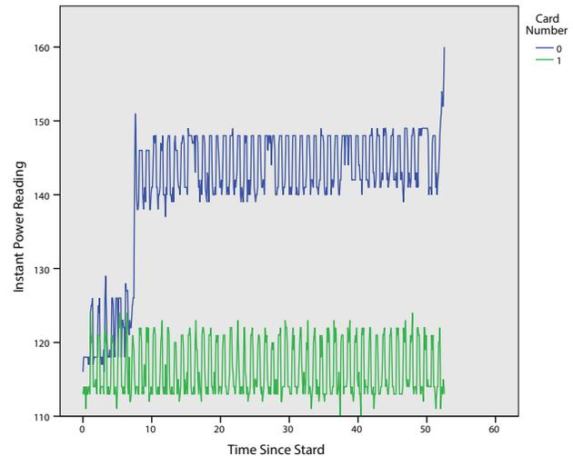
Fig. 7. Vector add workload on Xeon Phi without GeMTC. Shows power consumption of two cards. The workload was only offloaded to card number 0, the other card's data was left just to show that the up-down power curve exhibited in the sleep workloads is still present. After data generation is completed near the 10 second mark, power consumption quickly increases to the 140-150 Watt range staying there for the remainder of the computation.
