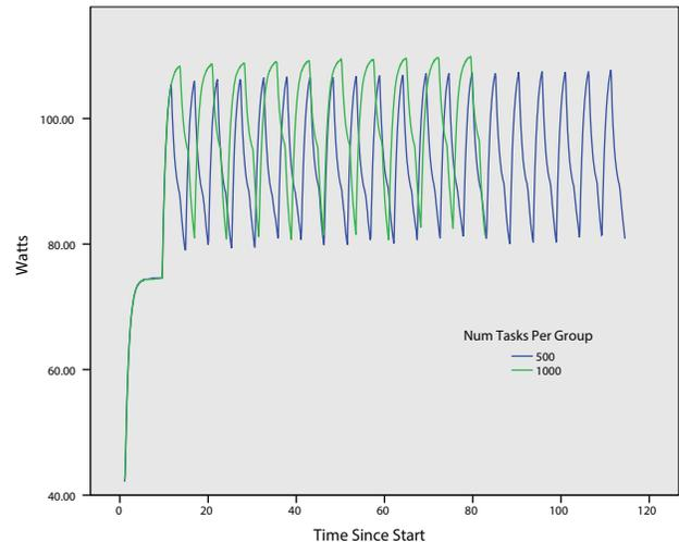
Fig. 4. Vector add implemented with GeMTC. Shows power consumption for two different workloads. For both we see that the power consumption follows a wave pattern increasing when the tasks are actually pushed to the device and decreasing as GeMTC waits for tasks to complete. 1000 tasks per group ultimately has a higher peak power consumption, but completes about 20 seconds quicker than 500 tasks per group.
