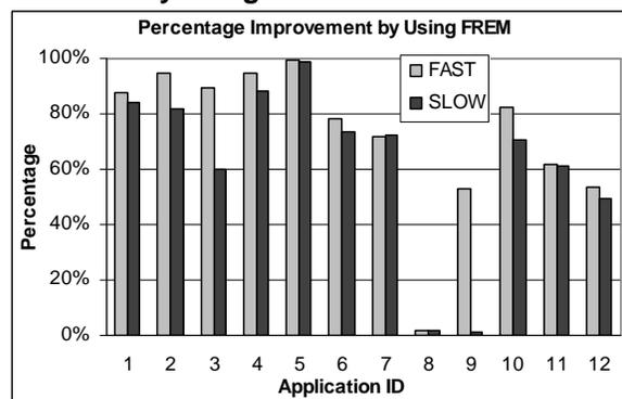
**Figure 5. Percentage improvement on restart latency by using FREM over BLCR**
