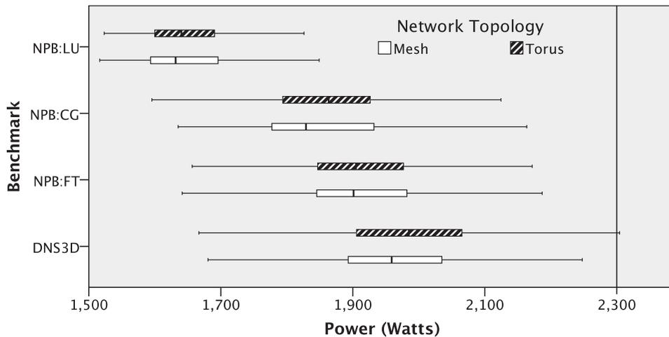
**Fig. 6.** Box plot comparison of average power consumption at the nodecard level for DNS3D and NPB benchmarks. Reference line at 2300 is mean power consumption of DGEMM, the most power hungry application we have profiled.
