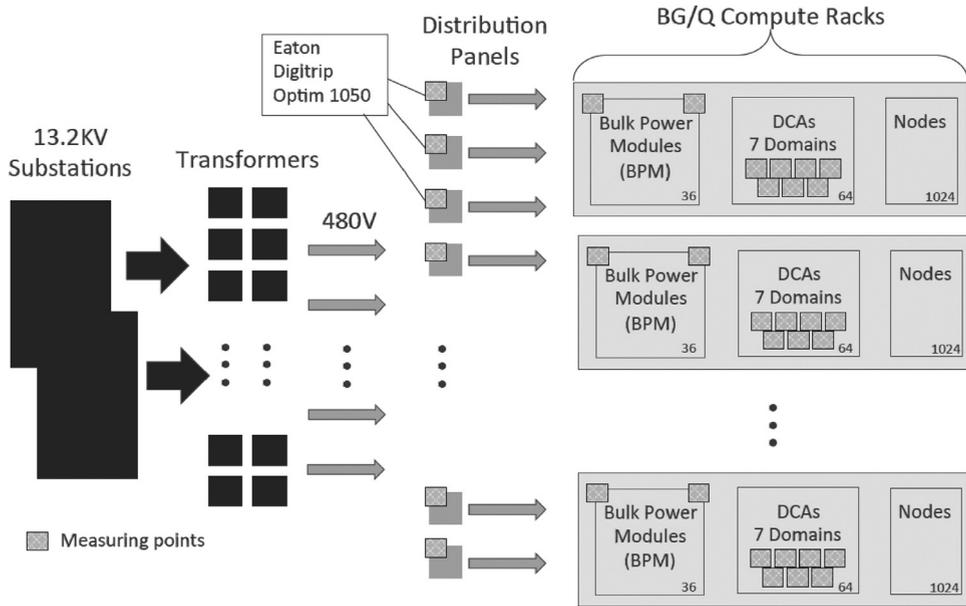
Fig. 1. Mira 480V compute power distribution system.
