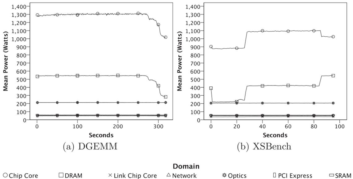
**Fig. 2.** Power profile of DGEMM run for about 5 min and XSBench run for about 2 min. While DGEMM shows relatively stable power consumption across all domains for the duration of the run, XSBench shows much more variation with two points of interest at 30 s when program starts generating data and 90 s when it switches from generation to random table lookups.
