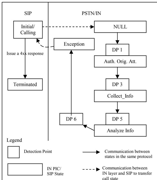
Figure 7: Partial mapping of SIP and PSTN/IN states
