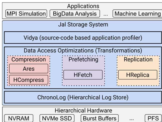
Figure 1: High-Level architecture of Jal Storage System
