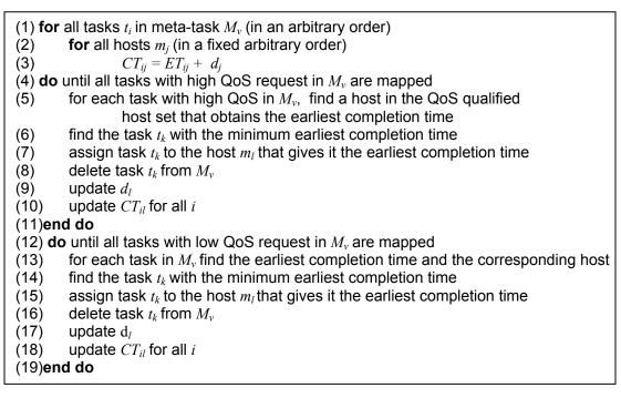
Fig. 2. The QoS Guided Min-Min heuristic
