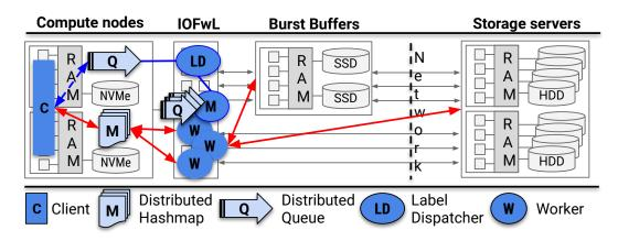
Fig. 6. Deployment example: LABIOS as I/O Forwarder Solution
