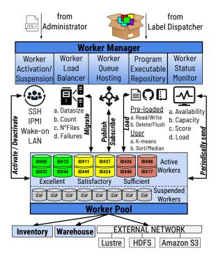
Fig. 4. LABIOS Server Internal Design.
