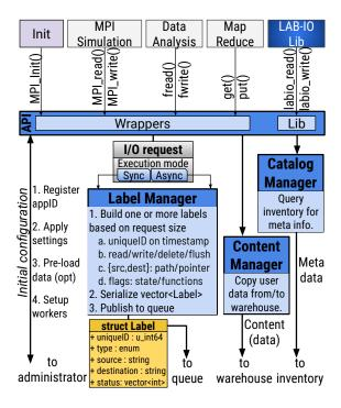
Fig. 2. LABIOS Client Internal Design.
