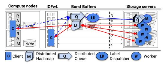
Fig. 8. Deployment example: LABIOS as Remore Distributed Storage
