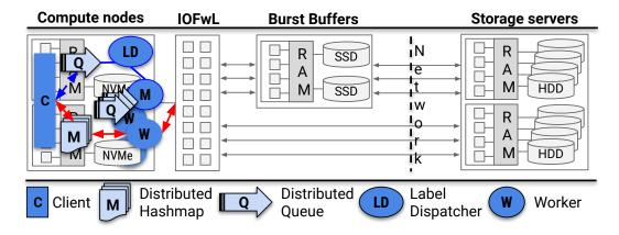
Fig. 5. Deployment example: LABIOS as I/O Accelerator in Compute Nodes
