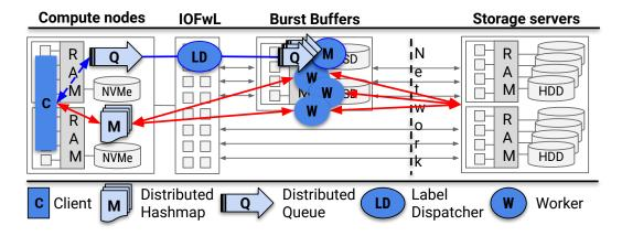
Fig. 7. Deployment example: LABIOS as I/O Buffering Platform
