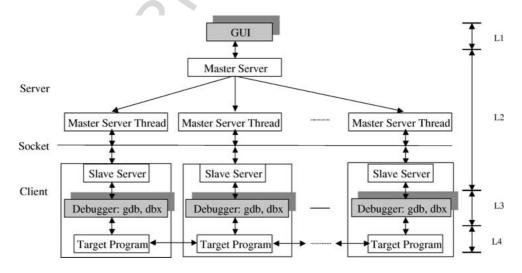
Figure 1. Architecture of the CDB. L1: graphical user interface level, L2: network communication level, L3: sequential debugger level, and L4: parallel and distributed program level.
