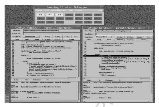
Figure 10. The CDB views for debugging MPI programs.
