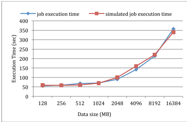
Figure 10. Performance comparison between HEC and YARNsim on Teragen benchmark: input data size varies from 128 MB to 16 GB; the number of nodes is 16.
