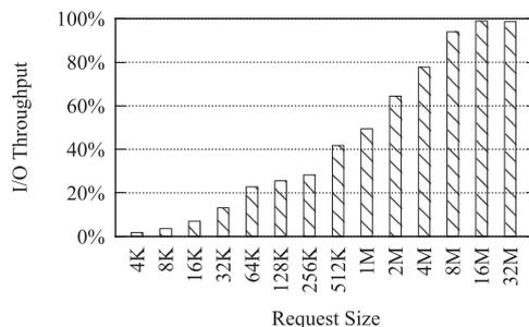
Fig. 1. I/O throughput normalized to the maximal system performance for random reads with different request sizes.
