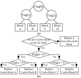
Figure 1: (a) Binary Tree-based PLRU replacement policy for one cache set in a 4-way set associative cache. (b) The process of searching a replacement candidate in the PLRU policy.
