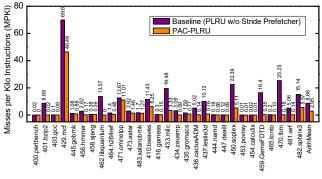
Figure 6: Misses per Kilo-Instructions (MPKI) of PAC-PLRU policy compared with a baseline system. L1 32K 4-way, L2 256K 8-way, MPKI results on L2 cache.
