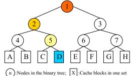
Figure 5: An example of behavior of the hash function for an 8-way set associative cache. The circles represent the nodes in the binary tree which has 3 levels and 7 nodes (No. 1 to 7). The rectangles represent the cache blocks in one cache set which has 8 blocks (A to H).
