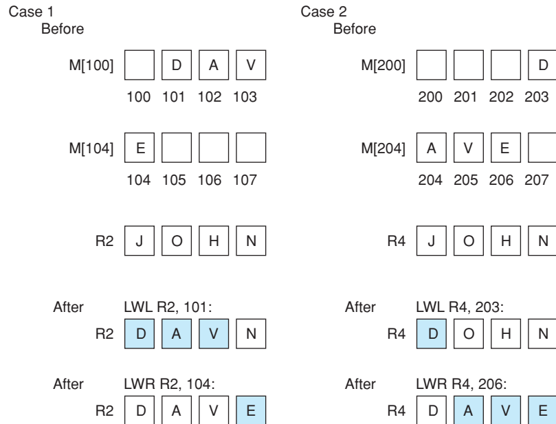
FIGURE D.7.1 MIPS instructions for unaligned word reads. This figure assumes operation in big-endian mode. Case 1 first loads the 3 bytes 101, 102, and 103 into the left of R2, leaving the least significant byte undisturbed. The following LWR simply loads byte 104 into the least significant byte of R2, leaving the other bytes of the register unchanged using LWL. Case 2 first loads byte 203 into the most significant byte of R4, and the following LWR loads the other 3 bytes of R4 from memory bytes 204, 205, and 206. LWL reads the word with the first byte from memory, shifts to the left to discard the unneeded byte(s), and changes only those bytes in Rd. The byte(s) transferred are from the first byte to the lowest-order byte of the word. The following LWR addresses the last byte, right-shifts to discard the unneeded byte(s), and finally changes only those bytes of Rd. The byte(s) transferred are from the last byte up to the highest-order byte of the word. Store word left (SWL) is simply the inverse of LWL, and store word right (SWR) is the inverse of LWR. Changing to little-endian mode flips which bytes are selected and discarded. (If big-little, left-right, load-store seem confusing, don't worry; they work!)
