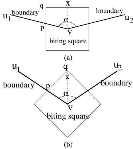
Figure 7 : The orientation of the biting-square: (a) if  $135^\circ \leq \alpha \leq 225^\circ$ , one side of the biting-square is aligned with  $vx$ . (b) if  $\alpha < 135^\circ$  or  $\alpha \geq 225^\circ$ , then the diagonal edge of the biting-square is aligned with  $vx$ .
