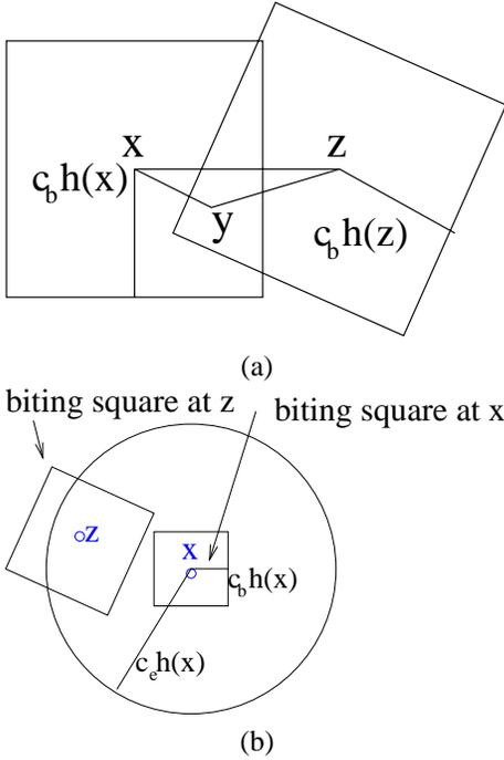
**Figure 9** : The biting-squares and packing-spheres. (a) a point  $y$  is covered by at least two biting-squares, (b) for any biting-square  $\Pi(x, c_b f(x))$ , there must exist a biting-square centered at  $z$ , such that  $z$  is contained inside the sphere  $B(x, c_e f(x))$ , where  $c_e = 2\sqrt{2}c_b / (1 - \sqrt{2}\alpha c_b)$ .
