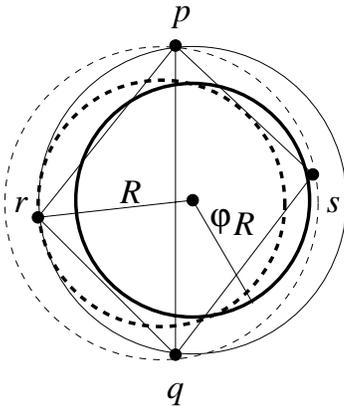
**Figure 13** : The shared edge  $pq$  of two triangles  $pqr$  and  $pqs$  are  $\phi$ -locally Delaunay. The dashed circles are the circumcircle and  $\phi$ -circumcircle of triangle  $\nabla pqs$ . And the solid circles are the circumcircle and  $\phi$ -circumcircle of triangle  $\nabla pqr$ . Notice that the edge  $pq$  is not locally Delaunay under classic Delaunay definition.
