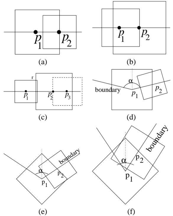
**Figure 11** : The configurations of adjacent biting centered at vertices of input boundary. Cases (a): the spacing at  $p_2$  is less than that of  $p_1$ ; (b): the spacing at  $p_2$  is larger than that of  $p_1$ ; (c):  $p_2$  is the intersection of  $\Pi(p_3, c_bf(p_3))$  with the boundary segment; (d):  $p_1$  is input vertex, and the input angle at  $p_1$  is larger than  $135^\circ$ . (e) and (f):  $p_1$  is input vertex, and the input angle at  $p_1$  is less than  $135^\circ$ .
