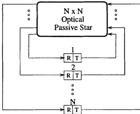
Fig. 1. An  $N$ -node optical passive star network.
