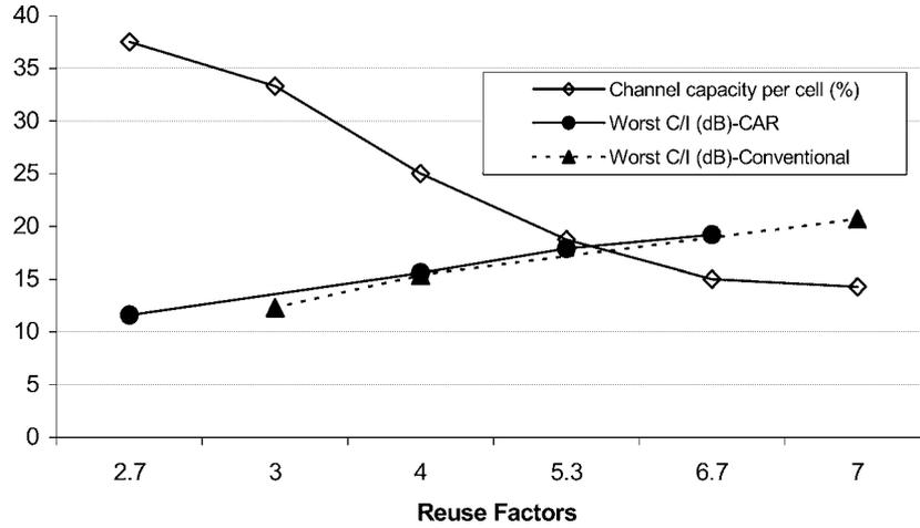
Figure 8. Performance comparisons between CAR  $N * (3 + 1)$  and conventional  $N * 3$  reuse plans utilizing wide-beam trisectorized cell with 3 dB, 13.5 dBd gain, 120-degree directional antenna.
