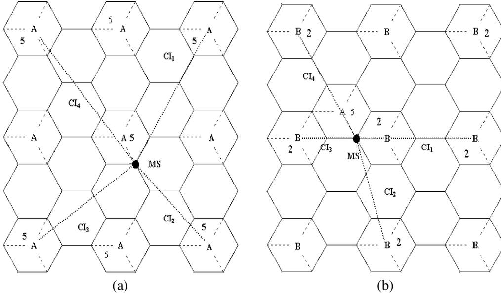
Figure 7. Worst interference location in  $4 * (3 + 1)$  reuse plan utilizing 120-degree wide-beam trisectorized cell. (a) Interference on sector S1 (channel 5). (b) Interference on sector S3 (channel 2).
