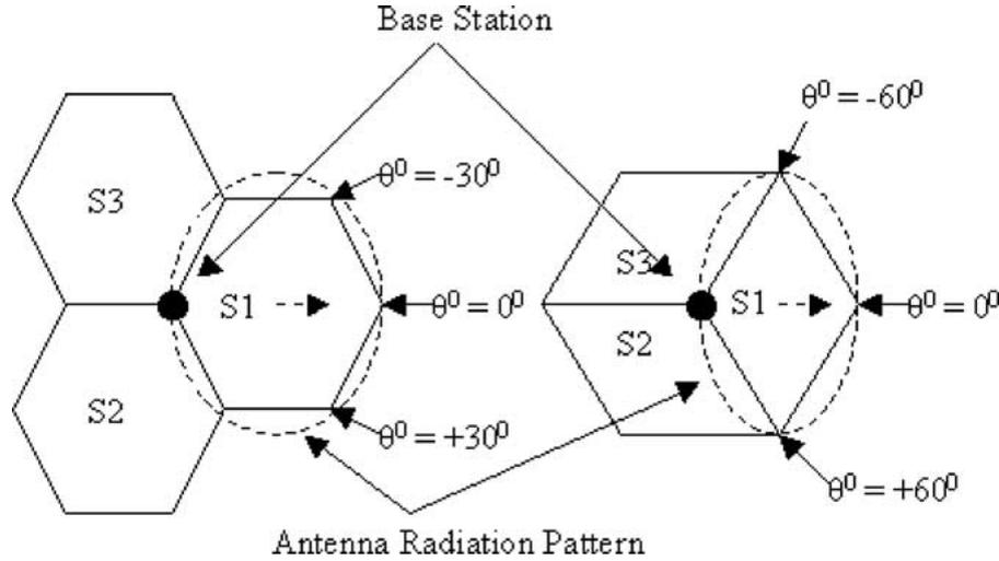
Figure 2. Cell layouts: Sector S1 is served by a directional antenna. Left: 60-degree narrow-beam trisectorized cell. Right: 120-degree wide-beam trisectorized cell.
