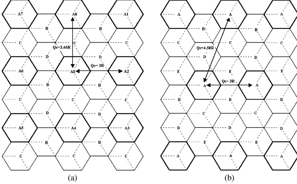
Figure 4. CAR cell reuse layouts and reuse distances for 4 and 5-cell reuse: (a)  $N = 4$ ; (b)  $N = 5$ .
