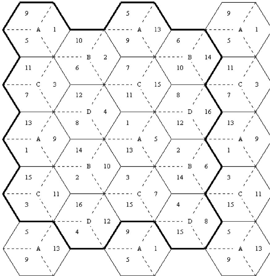
Figure 5. Repeat pattern for CAR  $4 * (3 + 1)$  reuse plan utilizing 120-degree wide-beam trisectorized cell.
