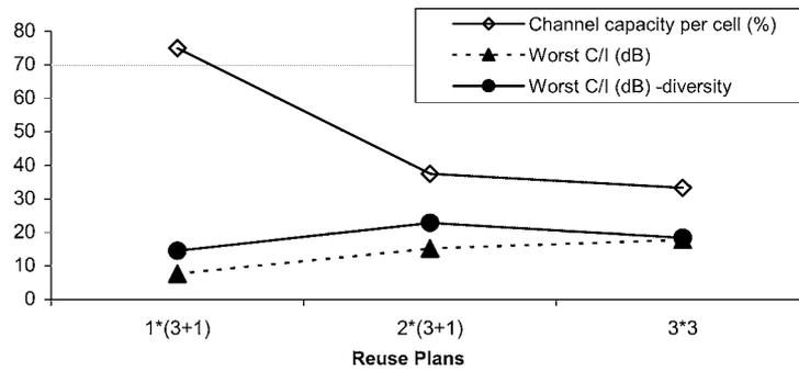
Figure 9. Performance comparisons between CAR  $N * (3 + 1)$  and conventional  $N * 3$  reuse plans utilizing narrow-beam trisectorized cell with 3 dB, 15 dBd gain, 65-degree directional antenna.
