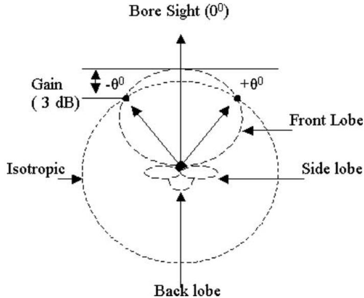
Figure 1. Directional antenna radiation pattern and antenna gain relative to omni-directional system.
