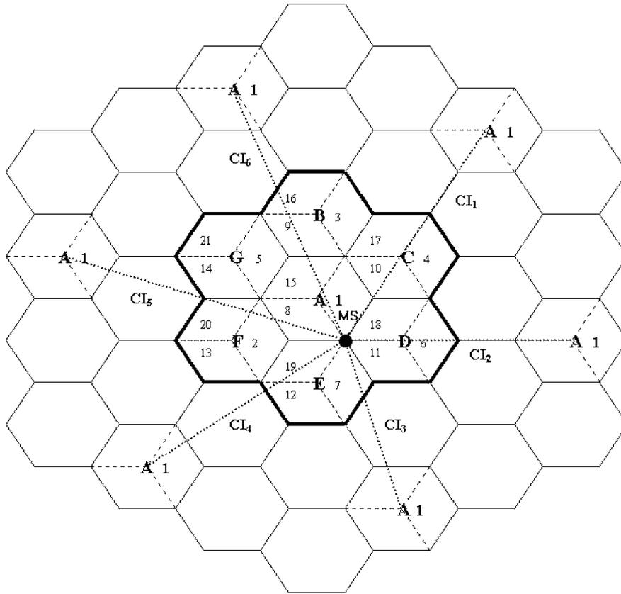
Figure 3. Conventional  $7 * 3$  reuse plan and worst co-channel interference scenario.
