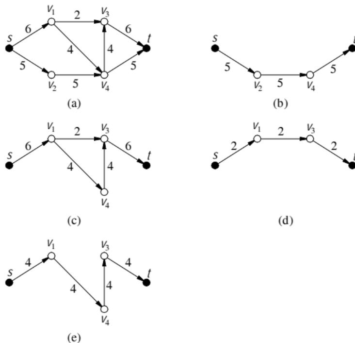
**Figure:** Any  $s - t$  flow of value  $L$  can be decomposed into at most  $|A|$   $s - t$  paths of total value  $L$  and possibly some circuits.
