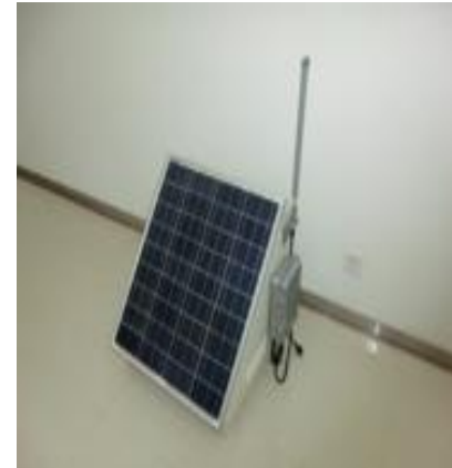
Mesh Nodes, Solar panel
