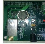
Fig. 6: The prototype of the wireless gas leak detection sensor node
