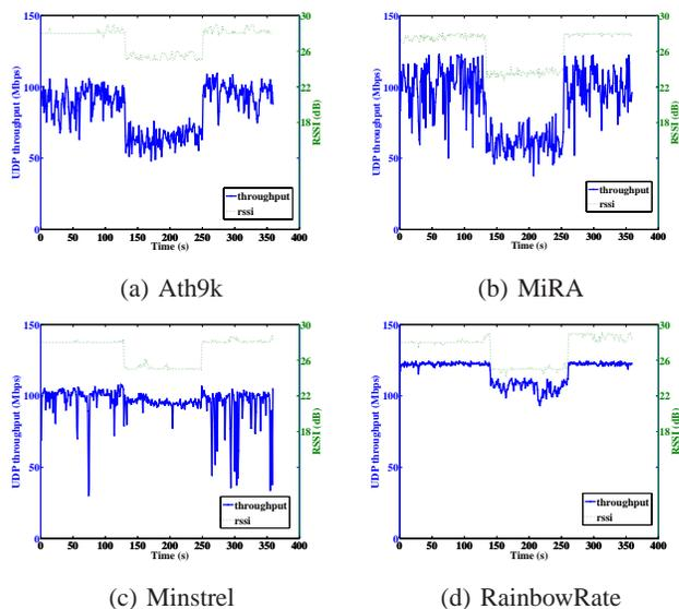
Fig. 6: RA UDP throughput with dynamic transmit powers.
