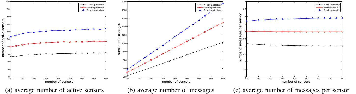
Fig. 4. Results for  $p$ -self-protection ( $p = 1, 2, 3$ ) when number of sensors increases from 100 to 500.
