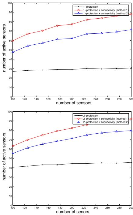
Fig. 5. Number of active sensors for  $p$ -self-protection with connectivity (Upper:  $p = 1$ ; Lower:  $p = 2$ ) when number of sensors increases.
