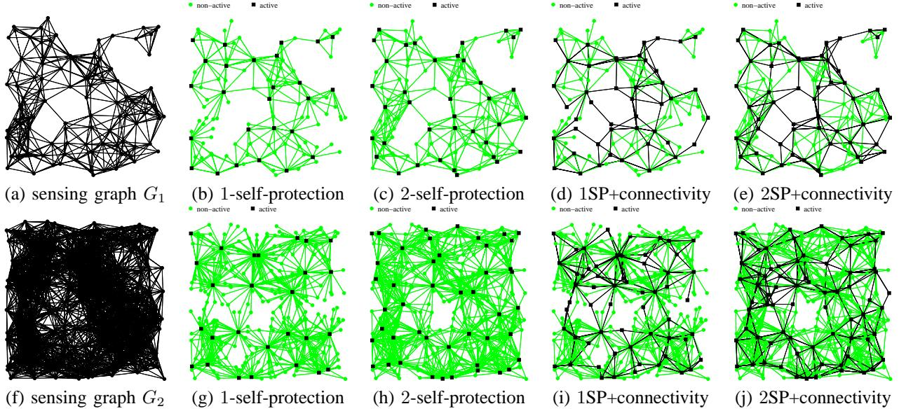
Fig. 3. Active sets generated by our self-protection algorithms for sensing graph  $G_1$  with 100 sensors and sensing graph  $G_2$  with 300 sensors. Here, black squares are active nodes and gray dots are non-active nodes. Black links in (d)(e)(i)(j) are links in the backbone keeping the active sensors connected.
