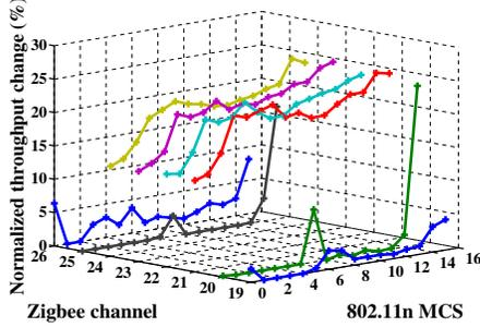
Fig. 3: Normalized 11n throughput degradation in the presence of 15.4 interference
