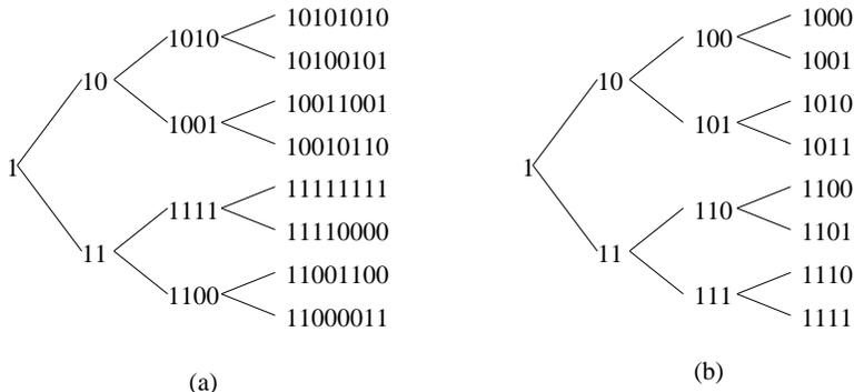
Figure 1: OVSF code: (a) code-tree structure; (b) binary color representation.
