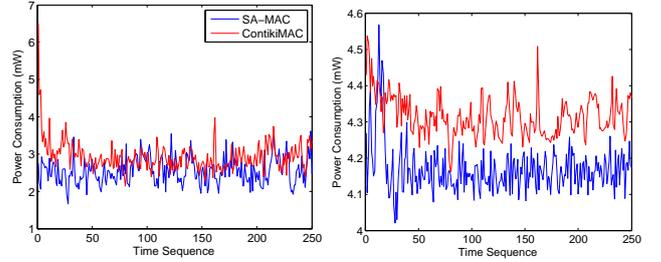
Fig. 13. Power Consumption in two protocols
