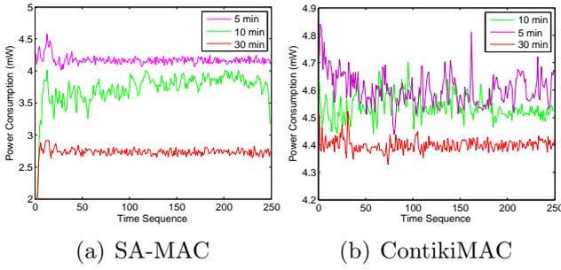
Fig. 14. Power Consumption in two protocols
