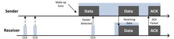
Fig. 6. Postpone waking up time: phase-lock.
