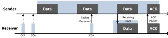
Fig. 1. ContikiMAC Mechanism
