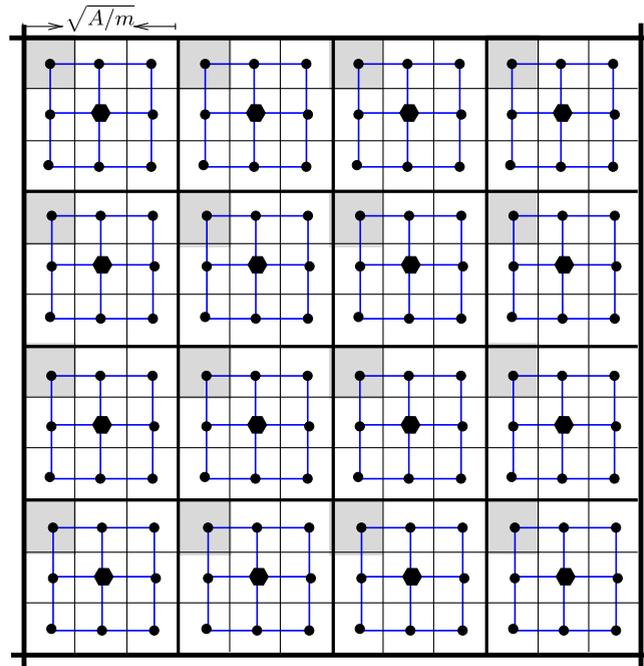
**Fig. 5.** Sparse backbones. The shaded cells can be scheduled simultaneously. In any time slot, there are exactly one link initiated from every activated station-cell.
