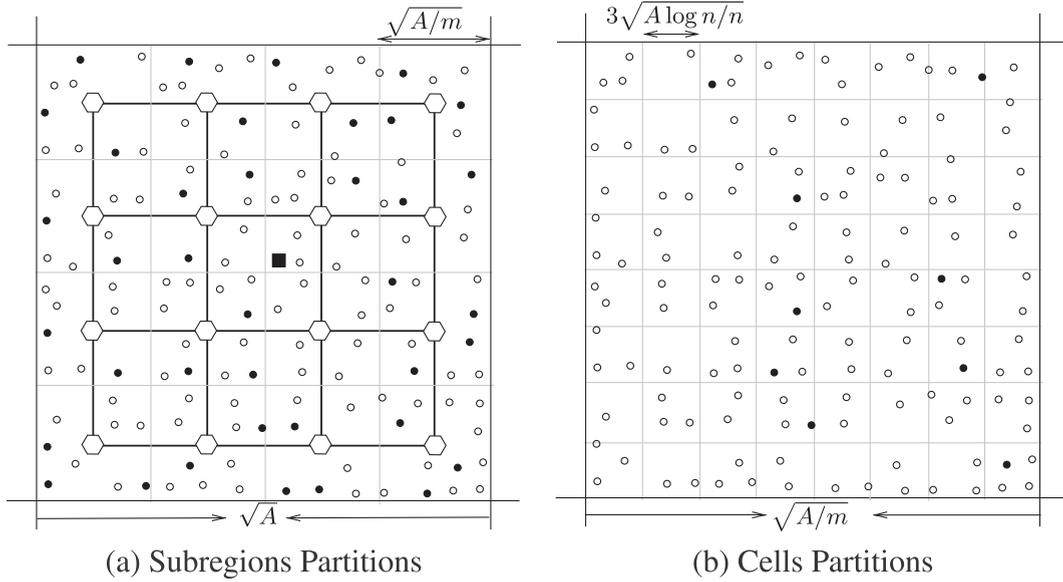
**Fig. 2.** The small hexagons are the BSs that are placed in the center positions of the subregions of area  $\frac{A}{m}$ . The shaded small square is the source of a given multicast session. The small circles are the ordinary ad hoc nodes, and the shaded circles are the destinations of the given multicast session.
