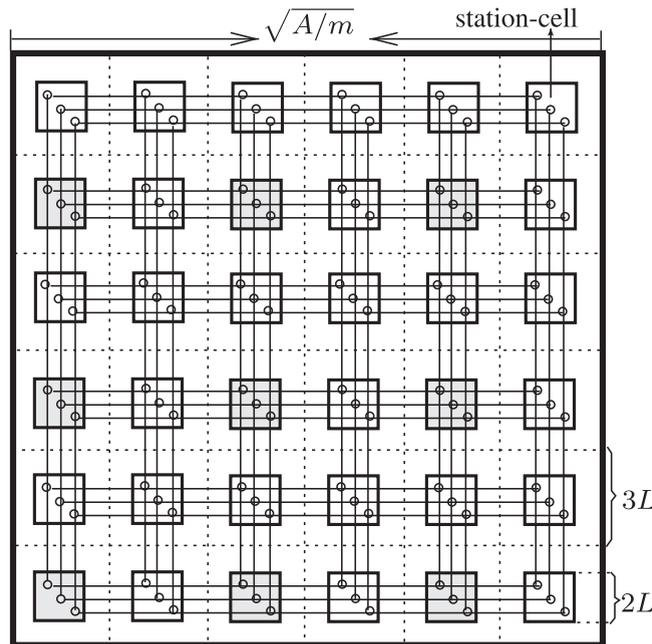
**Fig. 6.** Dense backbones. There is one station-cell centered at each cell of  $\mathbb{I}_i(\sqrt{A/m}, 3L)$ , where  $L = \sqrt{A \log n/n}$ . The shaded station-cells can be scheduled simultaneously. In any time slot, there are  $2 \log n$  concurrent links initiated from every activated station-cell.
