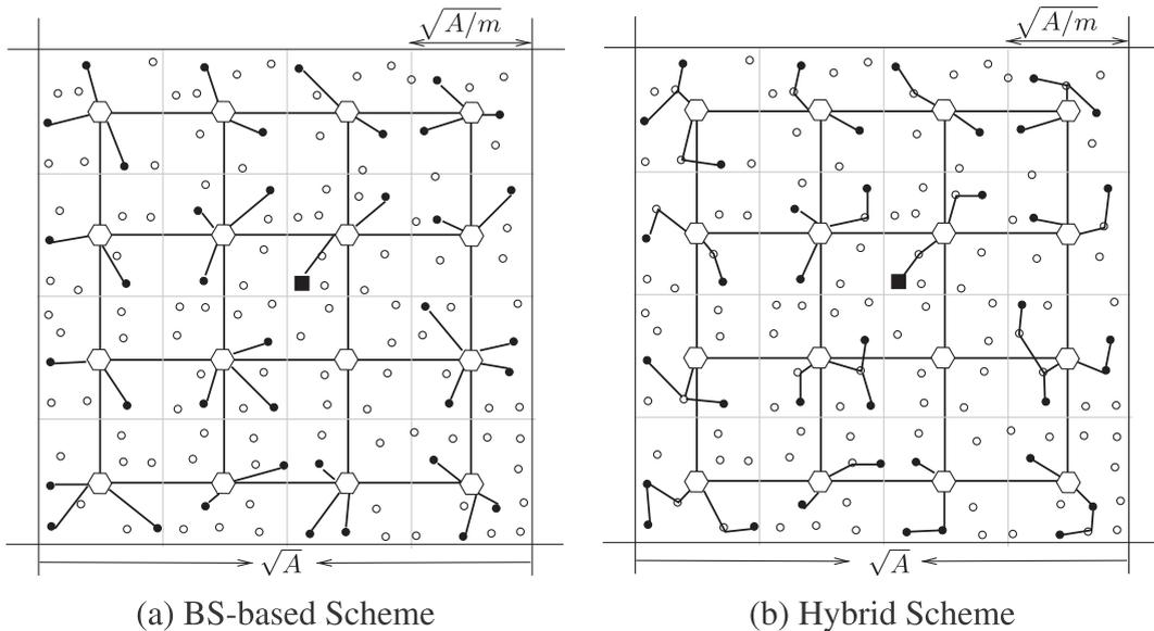
**Fig. 7.** Multicast schemes. (a) BS-based Scheme. The sources directly transmit data to BSs during the uplink phase and BSs also directly deliver received data to destinations during the downlink phase. (b) Hybrid Scheme. In each subregion, the data are transported to the BS by a multi-hop pattern. The communications between the ad hoc nodes in different subregions are relayed by the corresponding BSs.
