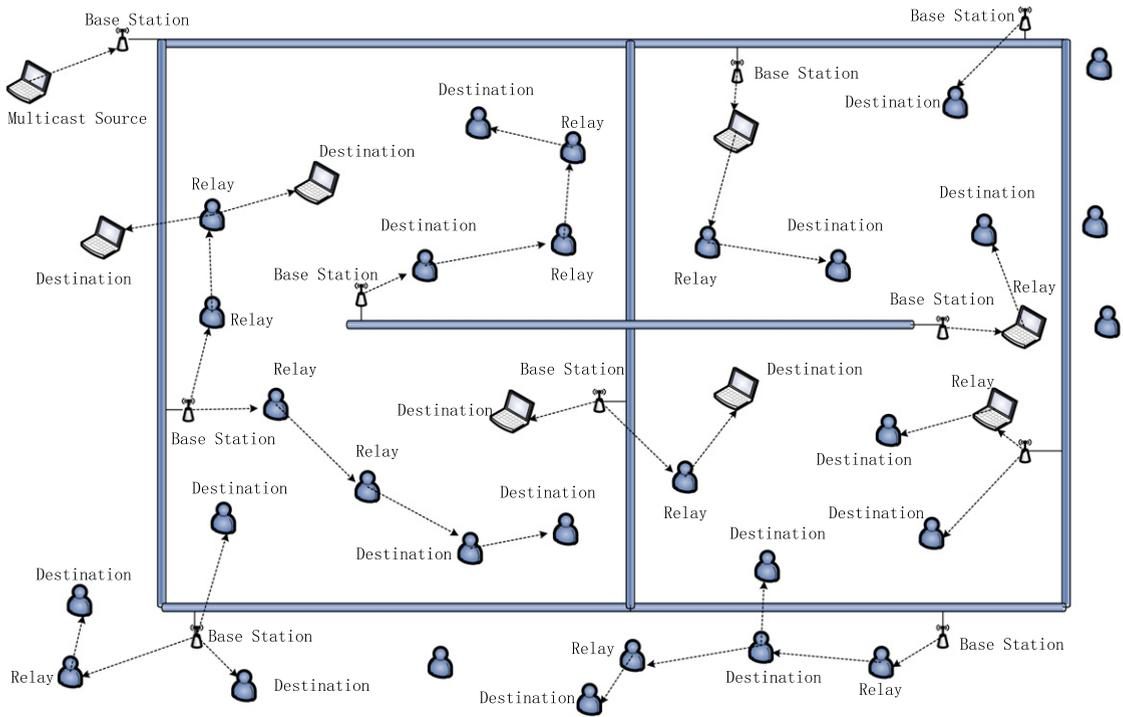
**Fig. 1.** An illustration of the multicast session in ad hoc networks with infrastructure support. Some of the users might be close to data sources (e.g., Internet access points), and they would act as sources for the multicast traffic. Other nodes would act as relays and sinks (destinations) for the data. The base stations are connected with links of high bandwidth (e.g., wired links).
