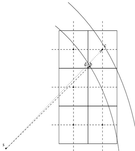
Figure 5: Point coverage. The grid is given by the dotted lines, and the solid lines separate and define the coverage areas of grid points.
