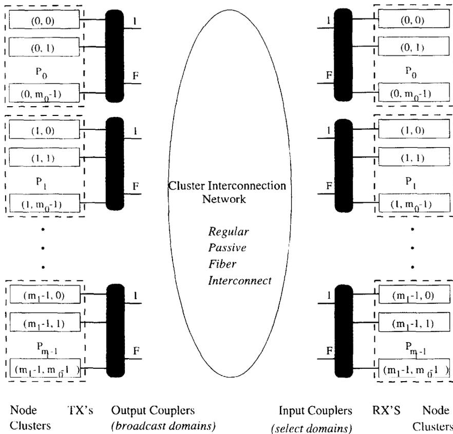
Fig. 1. Multi-sar network with discrete broadcast-select domains:  $m_1$  clusters, each with  $m_0$  nodes transmitting through output couplers and receiving through input couplers, interconnected via a regular CIN topology.
