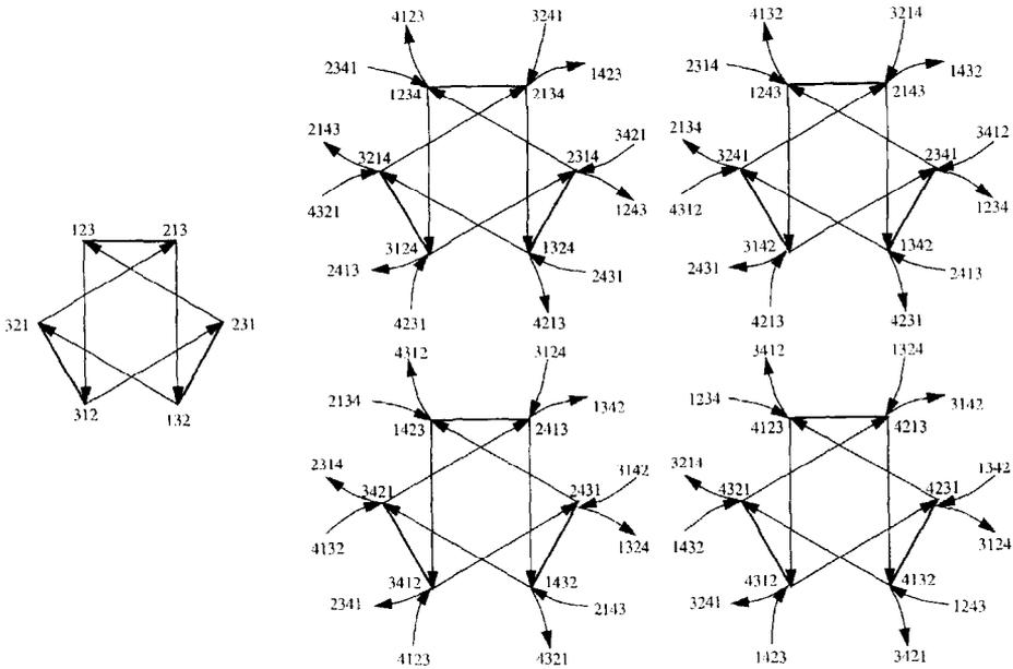
Fig. 3. The 3-dimensional and 4-dimensional right rotator digraphs.
