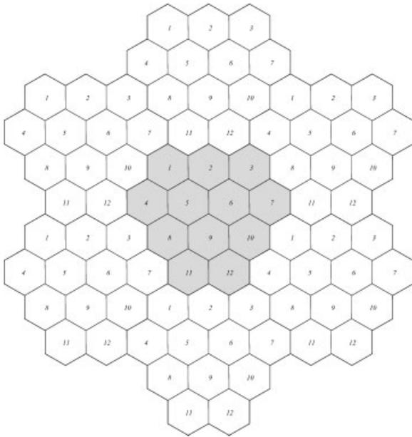
Fig. 9. Tiling of the plane into hexagons with 12 hexagons per cluster.
